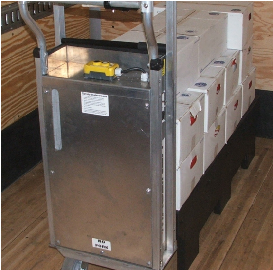
Figure 1: CooLift secured under a loaded pallet with the foot brake engaged
