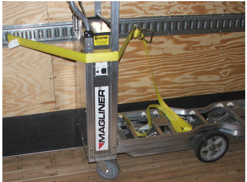
Figure 2: CooLift strapped into truck for transport
