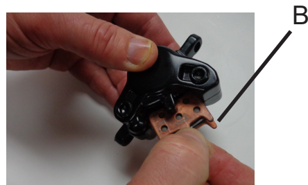
Figure 5 Inserting the pads
