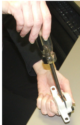
Figure 2 Compressing the piston
