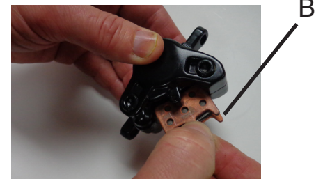
Figure 3 Removing/Inserting the pads
