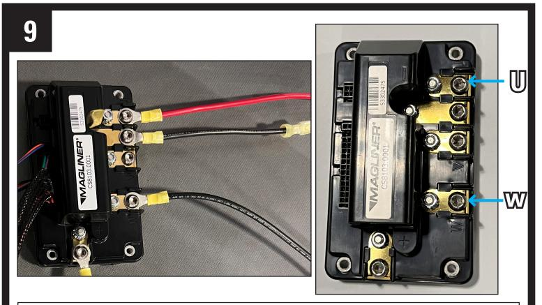
Connect the positive and negative wires as illustrated. (The red wire connects to the "U" slot and the black wire connects to "W" slot.
