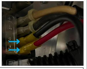
Locate the two existing Black and Red wires coming out of the motor. Trim the female contact terminals.
