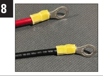
Attach the 61112 round end terminal to replace the female end connector. Crimp the connector to the wire as illustrated.
