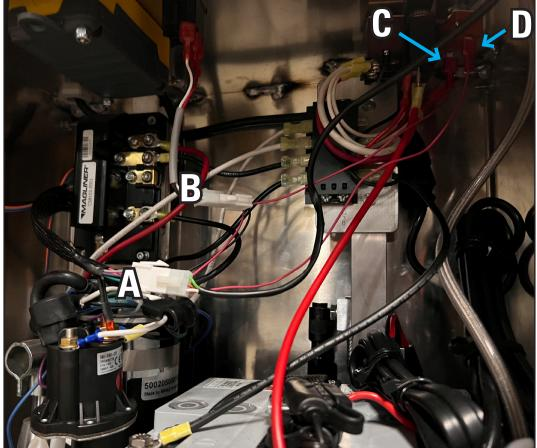
Connect connector "A" to the wire coming out of the throttle, "B" to the forward/reverse switch, "C" to the back end of the on/off propulsion switch and "D" to the front end of the on/off propulsion switch.
