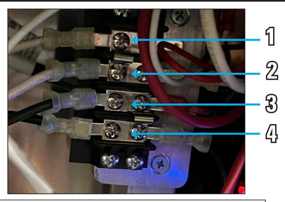
a.) Connect the top black wire from the controller to the 3rd terminal stripb.) Connect the bottom white wire from the controller to the 2nd terminal strip
