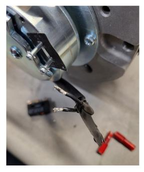
Crimp connectors onto the wires.
