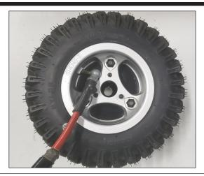
Install the (3) 80387 screws using the impact/drill and 5/16 Allen head socket. Inflate tire (max inflation 24 PSI).
