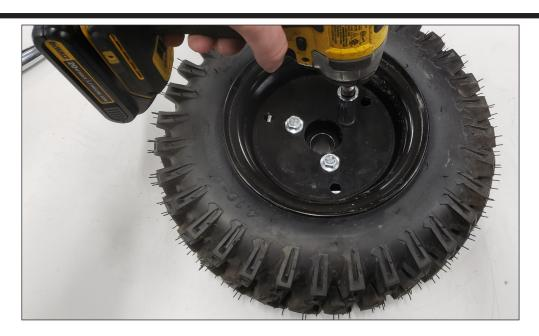
Use the impact/drill and  $1\!\!/2$ " socket to remove the (3) 80385 screws and the (3) 80630 nylon nuts. Remove inner wheel hub (from what had been the inside wheel).
