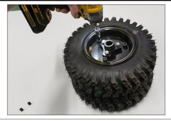
Use the impact/drill and the 5/16 Allen head socket to remove the (3) 80388 screws. Be sure to prevent the nuts from spinning on the opposite side.
