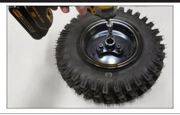
Fasten the wheel hub by installing the (3) 80386 screws previously removed in Step 6 using the impact/drill and 6mm Allen head socket.
