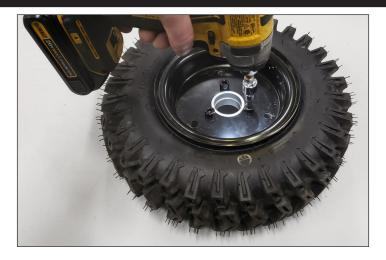
Use the impact/drill and 6mm Allen head socket to remove the (3) 80386 screws.
