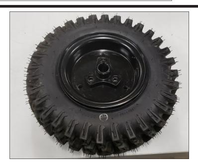
Insert wheel hub, aligning holes.
