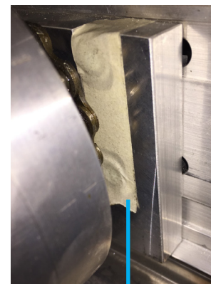
Tape can be used to keep lock nuts in place in the bearing mount plates.
