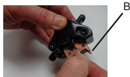
Figure 5 Inserting the pads
