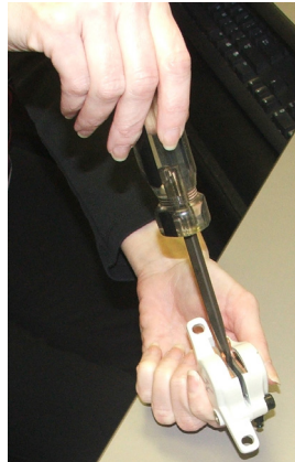
Figure 2 Compressing the piston
