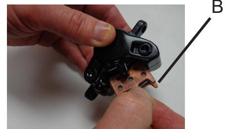
Figure 3 Removing/Inserting the pads
