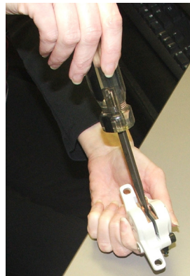
Figure 2 Compressing the piston
