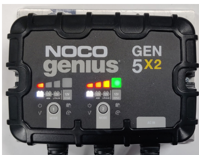
Normal Charging Lights
